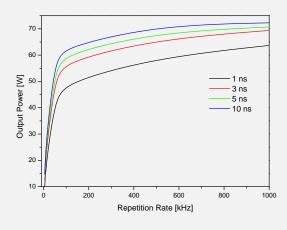
The lasers pulse duration can be changed by the seed laser and will additionally be formed by the gain dynamic of the amplifier stages. Therefore typical pulses will have a peak with a few nanosecond length followed by a declining tail with a changeable slope.
