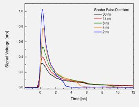
The rising edge of the pulse is determined by the gain of the amplifiers and can be manipulated to get pulse durations down to about 650 ps with a 2 ns input pulse. On the other hand the steepness can be flattened and the fullwidth half maximum duration variedby shaping the input pulse and therefore generate longer pulse durations.
