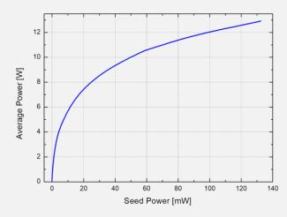
The modules are available in two versions, designed for different input power levels as a preamplifier or main amplifier module. With low seed powers of a few mW, the pre-amplifier used in double-pass configuration, provides a small signal gain of > 10.000 and already boosts the power to a few Watts (see left Figure).
