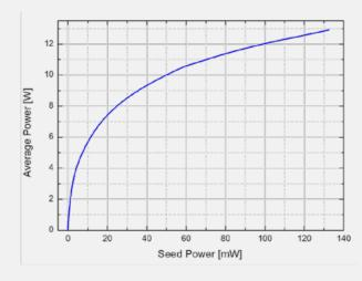
The modules are available in two versions, designed for different input power levels as a pre-amplifier or main amplifier module. With low seed powers of a few mW, the pre-amplifier used in double-pass configuration, provides a small signal gain of > 10.000 and already boosts the power to a few Watts (see left Figure).
