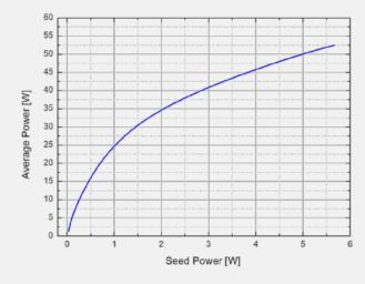
Due to the low nonlinearities, it supports > 50  $\mu$ J @ 700 fs without any stretching required and up to 1 mJ with only moderate chirp. With a fiber-based front-end providing 10 mW at 100 kHz, two stages are sufficient to reach an energy level beyond 500  $\mu$ J, boosting the energy by a factor of 5.000! A three stage design already show > 100 W output power and > 1 mJ pulse energy.
