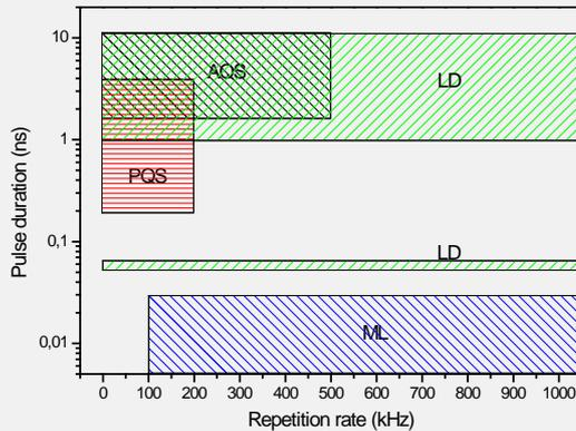
required pulse duration, active (AQS) and passive q-switched (PQS) oscillators, modulated laser diodes (LD) or pulse picked mode-locked oscillators (ML) are available on the market. The graphic shows an overview of the typical operation regimes for these lasers<sup>1</sup>.
