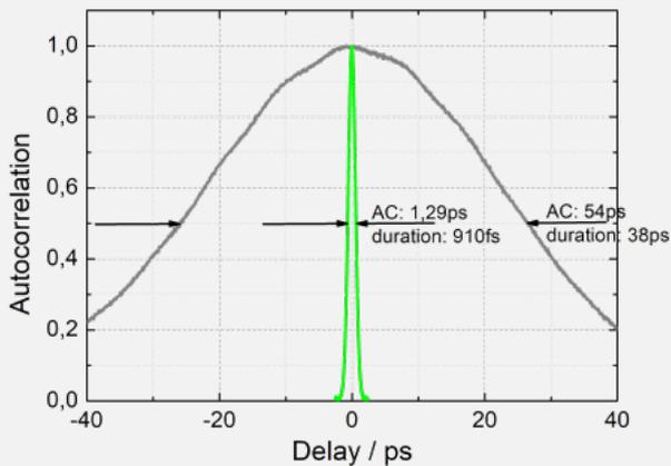
For two pulse durations the pulses use two different beam paths, of which one includes a grating compressor, which is matched to the seed laser. The switching is realized by a motorized half wave plate and a polarizer, such that also mixed states between the two regimes are also possible. The selected pulse durations have been measured to be 910 fs and 38 ps, respectively.
