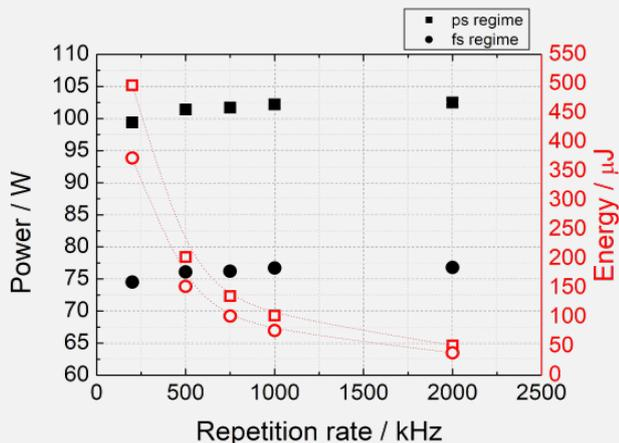
The output power of the system was measured to be > 100 W for repetition rates between 200 kHz and 2 MHz in the ps-regime. For femtosecond pulses, pulse energies of up to 350  $\mu\text{J}$  can be reached. The long term power stability was better than 0.5% RMS measured over a period of more than 12 hours.
