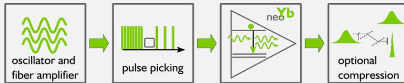
The system is based on a mode locked fiber oscillator, a pulse picker and up to three neoYb amplifier modules. The pulse duration can be selected by the used oscillator or by an optical switch when femto- and picoseconds pulses are applied.
